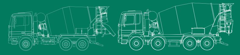
Drum walls made of high-strength wear resistant steel with a hardness of approx. 300 HB (Brinell)
